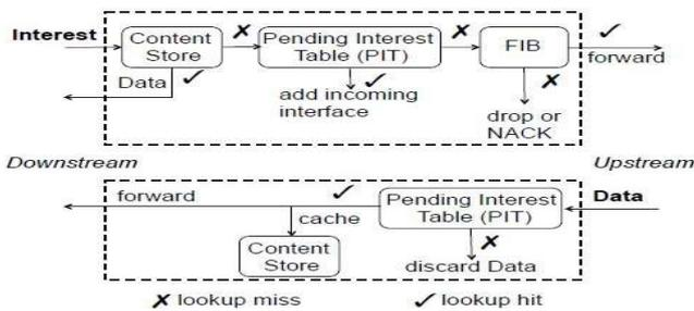
Fig. 2. Forward processing in NDN node [13]
