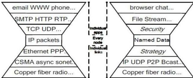
Fig. 1. Building blocks of the NDN architecture [18]
