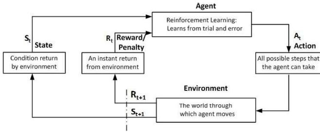
Fig. 2. Reinforcement Learning Model for Traffic Control System
